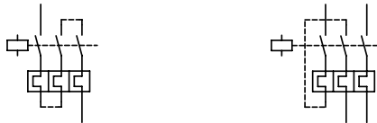
Figure 4: Wiring of the motor protection relay for the protection of AC or DC motors (bimetallic releases wired in series)
