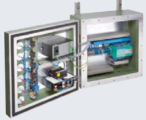
Control panel with intrinsic safety barriers in flameproof enclosure Ex d IIB for Zone 1
