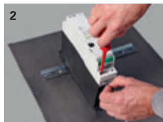
2 Connect mains and motor cables.
