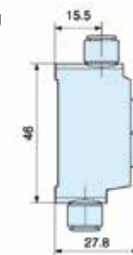
swivel elbow push-in connector 4 mm OD tube
