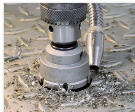
Drilling in checker sheet
