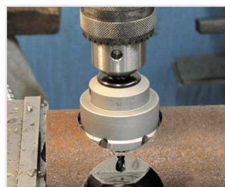
Drilling in pipes
