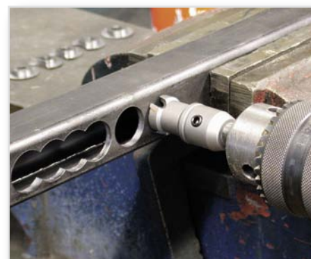
Drilling in square profiles
