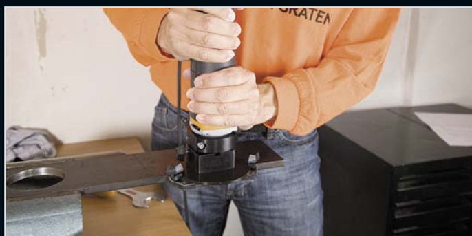
Initial drill-holes from: \varnothing 3.0 mm for pen cutters \varnothing 5.0 mm for spherical cutters
