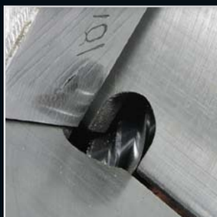
Exact deburring with self-generating milling cutter
