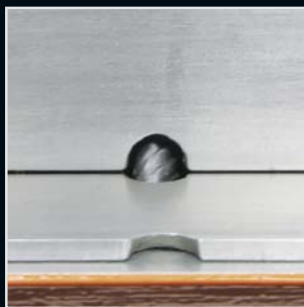
Position II: Material thickness from 1.5 mm
