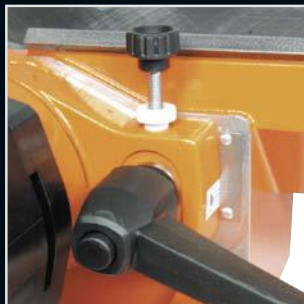
Fine adjustments to milling depth/ bevel width
