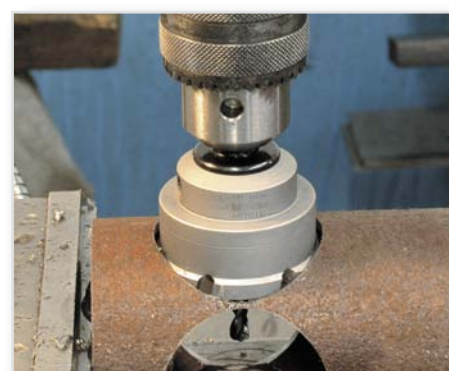
Drilling in pipes
