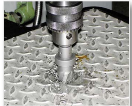
Drilling structured sheet metals
