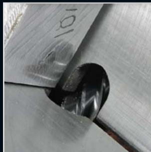
Exact deburring with self-generating milling cutter
