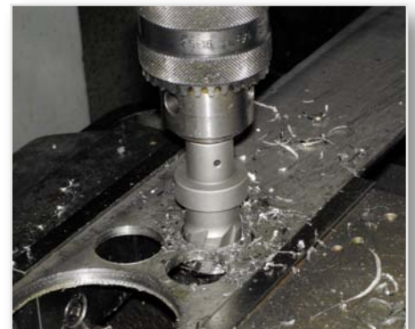
Drilling flat steels
