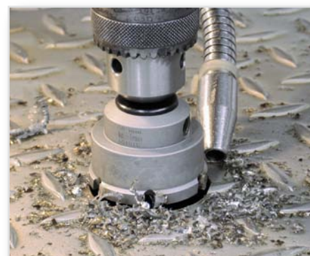
Drilling in checker sheet
