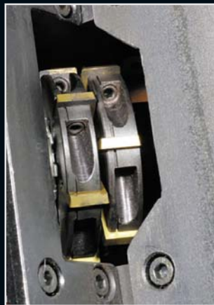
2 milling disks together with 6 inserts each
