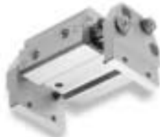
ACT-15-32 Long stroke, double acting w/magnetic piston
