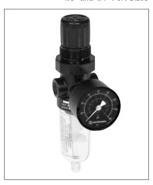
Ordering Information. Models listed include PTF threads, transparent bowl, relieving diaphragm, gauge, automatic drain, 5 µm element, 5 to 100 psig (0.3 to 7 bar) outlet pressure adjustment range\* .
