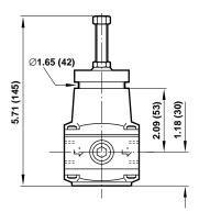
Panel mounting hole diameter: 1.65" (42 mm) Maximum panel thickness: 0.24" (6 mm)
