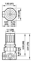
Panel mounting hole diameter: 1.19" (30 mm) Maximum panel thickness: 0.25" (6 mm)
