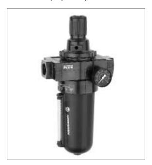
Ordering Information. Models listed include a 1 quart w/long element, yoke with PTF threads, knob adjustment, automatic drain, 40 µm element, relieving diaphragm, and a 5 to 120 psig (0.4 to 8 bar) outlet pressure adjustment range\*. A gauge is not included.
