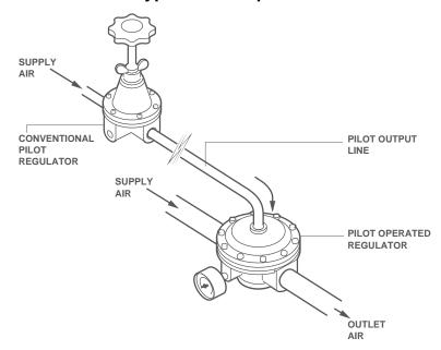
The pilot signal for the main regulator valve is usually onto a large diaphragm area. This results in pilot operated regulators having better regulation characteristics than spring operated general purpose regulators.
