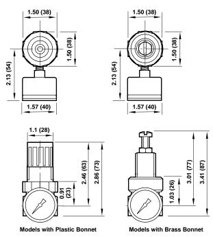
Panel mounting hole diameter: Models with plastic bonnet: 1.19" (30 mm) Models with brass bonnet: 0.81" (21mm) Maximum panel thickness: 0.25" (6 mm)
