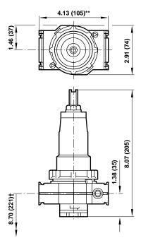
Panel mounting hole diameter: 2.06" (52 mm) Maximum panel thickness: 0.16" (4 mm) \*\* 6.18" (157 mm) for models with 3/4" ports
