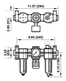
Alternative Micro-Fog Type G73A-Alternative Oil-Fog Type G73B-Includes lockout valve and Quikmount pipe adapter.
