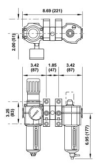
Alternative Micro-Fog Type E74K-Alternative Oil-Fog Type E74L-Includes Quikmount pipe adapters and porting block.
