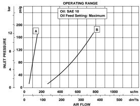
A: Minimum flow based on oil drip rate of 5 drops per minute. B: Maximum flow based on pressure drop of 5 psid (0.35 bar).
