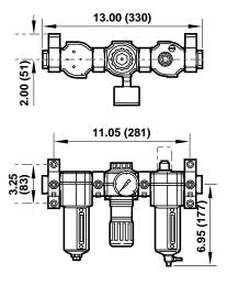
Alternative Micro-Fog Type G74A-Alternative Oil-Fog Type G74B-Includes Shutoff/Lockout valve and Quikmount pipe adapter.
