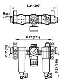
Alternative Micro-Fog Type G72A-Alternative Oil-Fog Type G72B-Includes Shutoff/Lockout valve and Quikmount pipe adapter. Shown with optional gauge and Quikclamp wall brackets.
