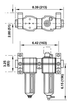
Alternative Micro-Fog Type G73C-Alternative Oil-Fog Type G73D-Includes lockout valve and Quikmount pipe adapter.
