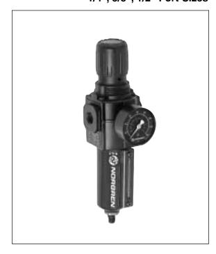
Ordering Information. Models listed include PTF threads, knob adjustment, automatic drain, metal bowl with liquid level indicator, 40 µm element, relieving diaphragm, 5 to 150 psig (0.3 to 10 bar) outlet pressure adjustment range\* with gauge.
