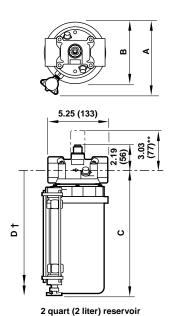
\*\* Optional pyrex sight-feed dome. † Minimum clearance required to remove bowl.
