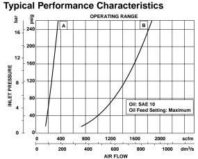
A: Minimum flow based on oil drip rate of 5 drops per minute. B: Maximum flow based on pressure drop of 5 psid (0.35 bar).
