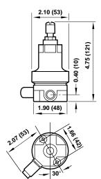
Mounting Holes (2 Places) 0.18" (4.6 mm) dia. by 0.39" (10 mm) deep. Use 10-32 thread forming screws.
