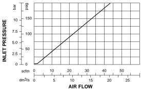
Fluid: Water Outlet Pressure: Atmoshpere Adjustment Knob: Full Open
