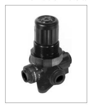
Ordering Information. Models listed include 10 mm push-in fittings, knob adjustment, relieving diaphragm, 0 to 70 psig (0 to 4.8 bar) outlet pressure adjustment range\* with gauge, with porting plug.
