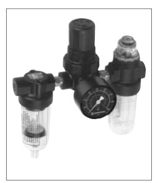
Ordering Information. Models listed include PTF threads, transparent bowls, filter with automatic drain, 5 µm element; regulator with relieving diaphragm, 5 to 100 psig (0.3 to 7 bar) outlet pressure adjustment range\*, gauge; lubricator with manual drain.
