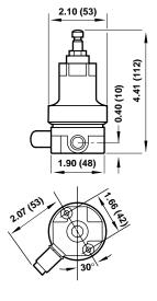
Mounting Holes (2 Places) 0.18" (4.6mm) dia. by 0.39 (10mm) deep. Use 10-32 thread forming screws.
