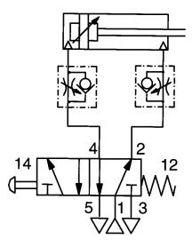
Figure 1. Typical valve/cylinder/flow control circuit If the cylinder selected had a 1/2" pipe port, most installers would apply 1/2" flow controls, 1/2" pipe and fittings, a 1/2" valve, and quite possibly, a 1/2" FRL! This approach leads to oversized, high priced components and higher long term operating compressed air costs over the life of the equipment. As a result, oversizing components occurs frequently and quickly leads to another popular pneumatic myth.
