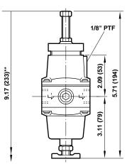
\*\* Minimum clearance required to remove bowl. Panel mounting hole diameter: 1.65" (42 mm) Maximum panel thickness: 0.24" (6 mm)
