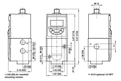
All units shipped with M12 five pin electrical connectors with interface for manifold mounting.
