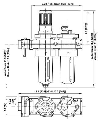
† Reduces by .16 (4mm) with knob in locked position. Add .15 (37mm) for unit with T-handle.
