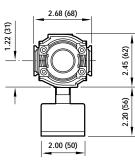
Panel mounting hole diameter 1.89" (48 mm) Panel thickness: 0.25 (6 mm)
