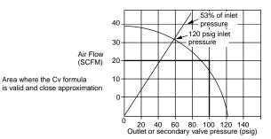
Example 1: Find air flow Q (scfm) if C<sub>V</sub> is known  $C_V$  (from valve catalog) = 1.8 Primary pressure p1 = 90 psig Pressure drop across valve  $\Delta P = 5$  psid
