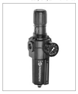
Ordering Information. Models listed include PTF threads, knob adjustment, automatic drain, metal bowl with liquid level indicator, 40 µm element, relieving diaphragm, 5 to 150 psig (0.3 to 10 bar) outlet pressure adjustment range\*, with gauge.
