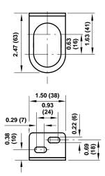
11-002 Bracket 11-008 Bracket (Units with 1/2" Ports) (18-001-003)
