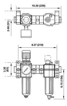
Alternative Micro-Fog Type D73K-Alternative Oil-Fog Type D73L-Includes lockout valve and porting block.
