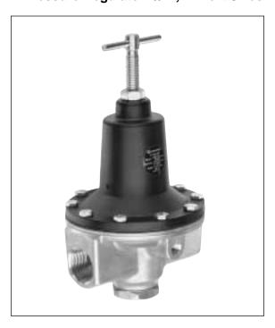
**Ordering Information.** Models listed have PTF threads, T-bar adjustment, non-relieving diaphragm, and 5 to 125 psig (0.3 to 8.5 bar) outlet pressure adjustment range\*. A gauge is not included.
