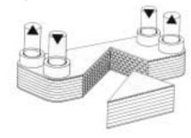
Corrugated stainless steel plates brazed with copper alloy into a honeycomb system create counter flow paths in both the air-to-air and air-to-refrigerant sides. Compressed air and refrigerant are securely contained in their separate channels to avoid leakage. The smooth flow path design provides a continuous cleaning action to retard oil and varnish buildup. These heat exchangers can be back-flushed for thorough cleaning when necessary.
