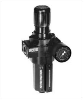
Ordering Information. Models listed include PTF threads, knob adjustment, automatic drain, metal bowl, 40 µm element, relieving diaphragm, 5 to 150 psig (0.3 to 10 bar) outlet pressure adjustment range\* with gauge.
