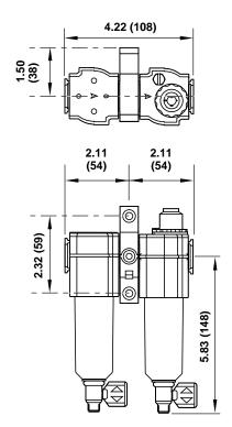
Alternative Micro-Fog Type D72C-Alternative Oil-Fog Type D72D-Includes Shutoff/Lockout valve.
