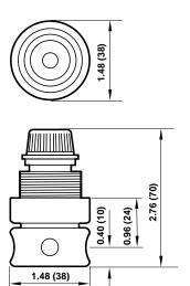
Panel mounting hole diameter: 1.19" (30 mm)
