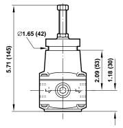
Panel mounting hole diameter: 1.65" (42 mm) Panel thickness: 0" to 0.24" (0 to 6 mm)
