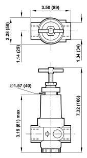
Panel mounting hole diameter: 1.65" (42 mm) Maximum Panel thickness: 0.37" (9.5 mm)
