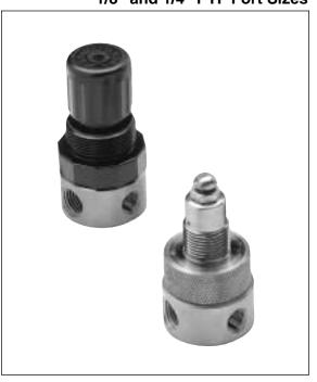
Ordering Information. Models listed include PTF threads, plastic bonnet with knob adjustment, non-relieving diaphragm, 5 to 100 psig (0.3 to 7 bar) outlet pressure adjustment range†, and without gauge.
