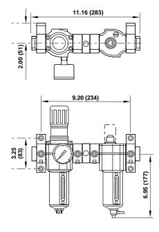
Alternative Micro-Fog Type D74K-Alternative Oil-Fog Type D74L-Includes lockout valve and porting block.
