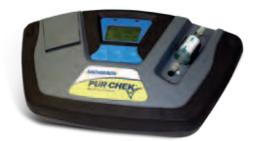
Pur • Chek™ is smarter and faster than any refrigerant identifier used in the industry today. Its compact size and ergonomic design makes testing easy and it utilizes non-dispersive infrared (NDIR) technology to determine the weight concentrations of R12, R134A, R22, hydrocarbons, and air. It also features 'Blend-Chek' analytical software which quickly and accurately indicates the presence of R410A blend refrigerant.
