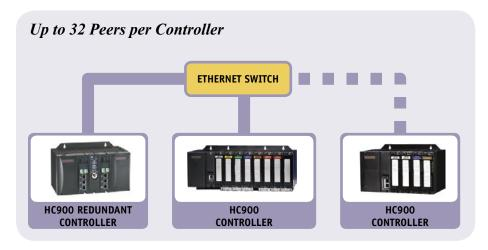
from simple loop control to interactive cascade, ratio, duplex, feed forward, three position step or custom control strategies. Auto tuning is standard on every control loop using Honeywell's proven "Accutunelll" tuning algorithm to reduce startup time and ensure on-spec product.
