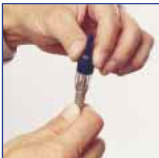
Interchangeable sensor tips can be swapped quickly and easily in seconds.
