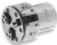
ACT-15-29 Three jaw, double acting w/magnetic piston
