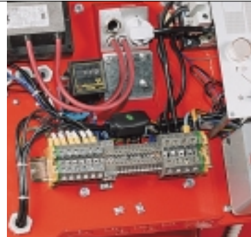
Example of the terminal board for electrical connections for P 140-200-300-450 T/N models
