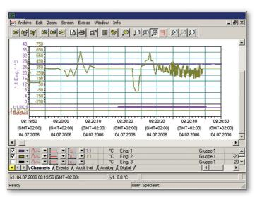
DataVU works with PC Evaluation Software (PCA3000), a program which runs under Windows 2000/XP/Vista and Windows 7. It can be used to manage, archive, visualise and evaluate the recorder data. Data from multiple and differently configured instruments is recognized by the PC Evaluation Software and stored in an archive database for future evaluation and traceability.
