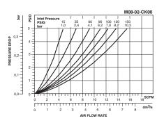
Flow data based on inlet pressure = 150 psig, 3 psid
