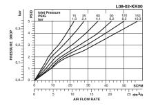
Flow data based on inlet pressure = 150 psig, 5 psid
