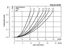
Flow data based on inlet pressure = 150 psig, 5 psid
