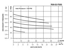
Flow data based on inlet pressure = 100 psig, secondary pressure 90 psig
