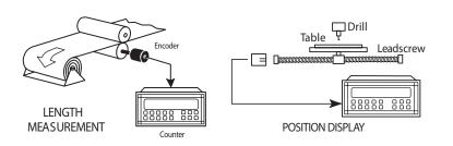
Applications: With the versatility of the VersaCount, just about any process can be monitored and controlled. Whether it is length measurement for the textile, metal or paper industries, position monitoring for metal fabrication or electronics, batch counting for product packaging, volume measurement for the beverage industry, shift monitoring for production lines, or range signaling for parking garages. Any process requiring timing, measuring or counting.
