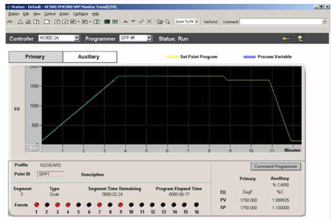
HC900 SP programmer trend display with a pre-plotted profile
