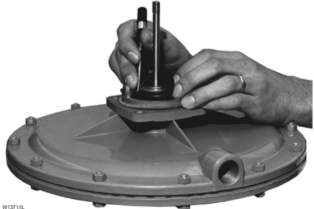
Figure 6. Installing Balancing Diaphragm. The Side of Diaphragm Marked PISTON SIDE Must Face Casing.
