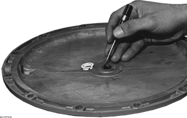
Figure 5. Inspecting Guide Bushing and Stem Seal O-Ring
