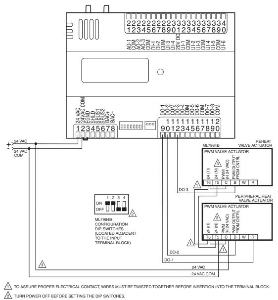
A MAKE SURE ALL TRANSFORMER/POWER WIRING IS AS SHOWN: REVERSING TERMINATIONS WILL RESULT IN EQUIPMENT MALFUNCTION.
