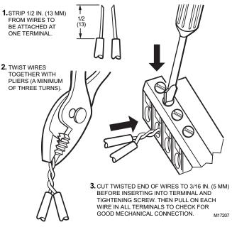
Fig. 14. Attaching two or more wires at terminal blocks.
