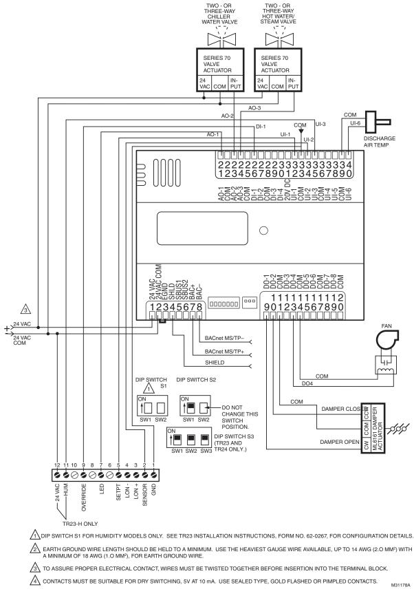
Fig. 22. Controller wiring diagram (model PUB6438S shown) with 4 to 20 mA heating, cooling, and model ML6161 damper actuator. (For note 2, refer to Fig. 14.)
