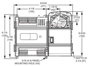
NOTE: CONTROLLER CAN BE MOUNTED IN ANY ORIENTATION. M31532
