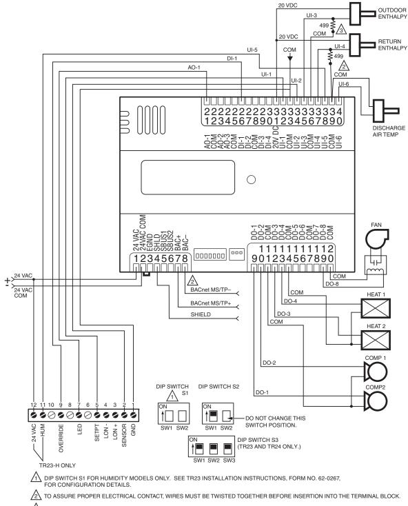
CONTACTS MUST BE SUITABLE FOR DRY SWITCHING, 5V AT 10 MA. USE SEALED TYPE, GOLD FLASHED OR PIMPLED CONTACTS.
