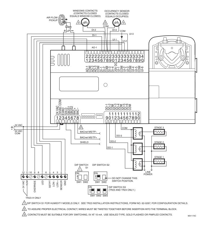
Fig. 18. Controller wiring diagram (model PVB6436AS shown) for typical VAV application with staged reheat. (For note 2, refer to Fig. 14.)
