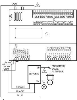
LT USE 1/4 IN (6 MM) PNEUMATIC TUBING. MINIMUM BRANCH LINE MUST BE 6 FT. (1.8M) OR LONGER.
