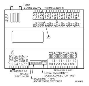
Fig. 24. LED, service, and network connection locations.
