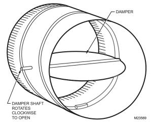
Fig. 2. Damper with 90 degree CW rotation to open.
