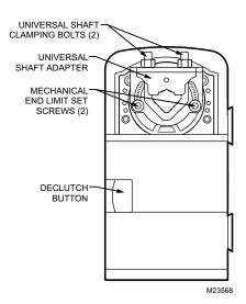
Fig. 1. Series 60 Floating Actuator.
