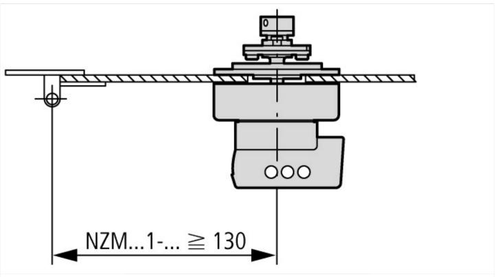
Minimum door coupling rotary handle clearance from door pivot point
