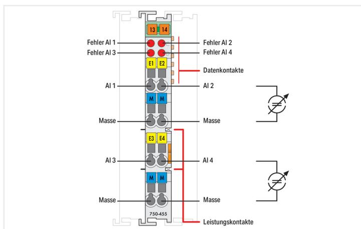
This analog input module processes standard 4–20 V signals.
