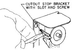
Fig. 5 — The controls have a screw type cutout stop. The stop screw must be loosened and moved to the stop setting desired. Tighten screw after setting is made.
