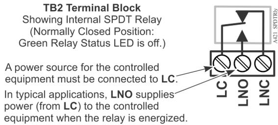
Figure 4 shows how to wire the A421 Control to use the same power source that powers the controlled equipment to also power the A421 Control.
